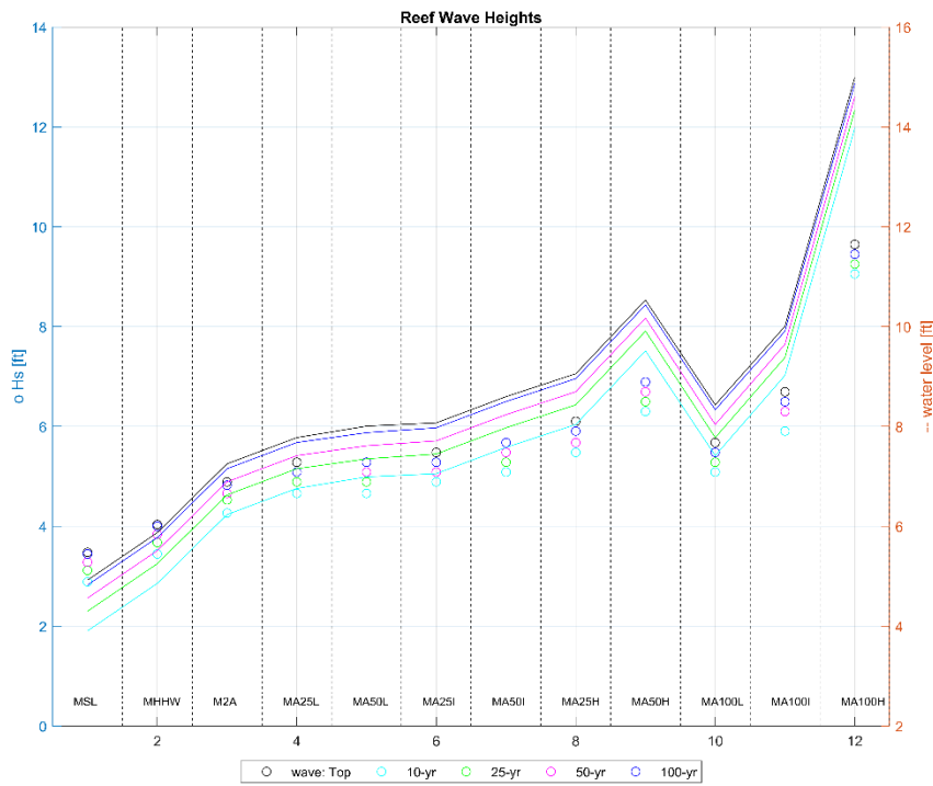
Figure 19. Maximum model outputs along the reef edge transect, Significant wave height in feet is shown on the left y-axis, and water elevation (feet) is shown on the right y-axis.
