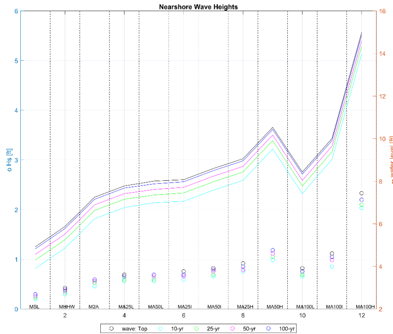
Figure 20. maximum model outputs along the nearshore transect, Significant wave height is shown on the left y-axis, and water elevation is shown on the right y-axis.
