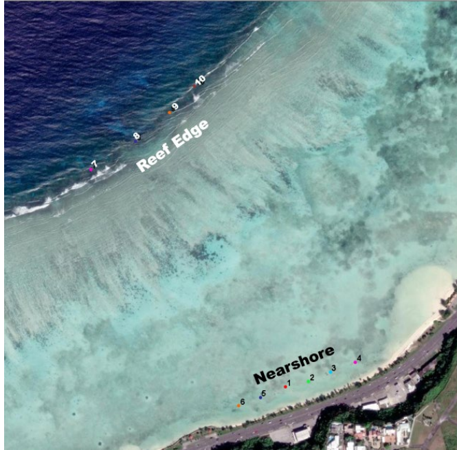
Figure 14. Location of the two-observation point transects for wave height ( H_s ) outputs from STWAVE
